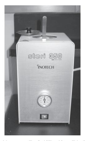
Fig. 2. Inotech instrument sterilizer Steri 350 used for sterilizing dissecting tools.
